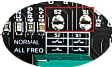
The factory default is not short circuited, which is the normal mode. The stereo output does not include the bass part below 200Hz.
